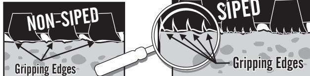
Research has shown that the most effective braking power occurs immediately prior to losing traction. Siping extends the window allowed for maximum braking power by giving the existing tread a helping hand. In the examples above notice how the SIPED tire has dozens more gripping edges. These micro edges reduce the distance needed for braking on wet and snow packed roads.
